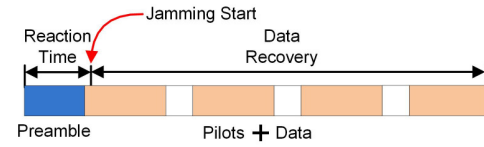
Fig. 5: Extended frame structure
