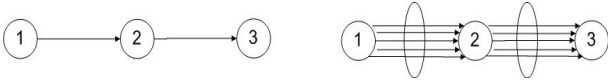
Fig. 2: two-link tandem network. Left: packet level queueing network; right: symbol level multi-queueing network.
