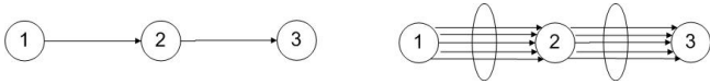
Fig. 2. two-link tandem network. Left: packet level queueing network; right: symbol level multi-queueing network.
